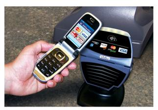
Near Field Communication (NFC), is a short-range, high frequency and low power wireless communication system. This technology, through the use of magnetic induction, creates a radio-wave field that allows for the exchange of data between two devices at a short range (usually 4 cm or less). Essentially, there is an active device (which acts as a reader) and a passive device (which acts as a tag). The reader generates a radio frequency (RF) field that checks the immediate area for nearby tags.
